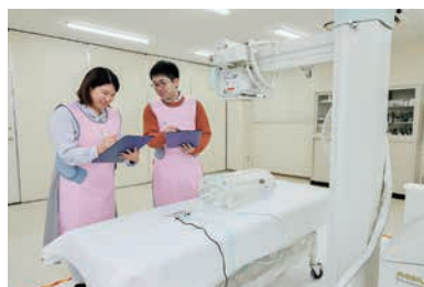
Exercise to measure radiation dose from X-ray irradiation
